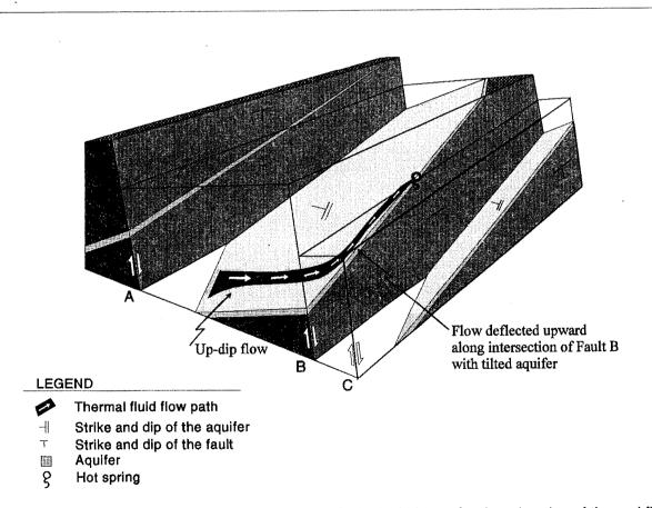
Figure 1: Block diagram illustrating the tilted fault block theory for the migration of thermal fluid
