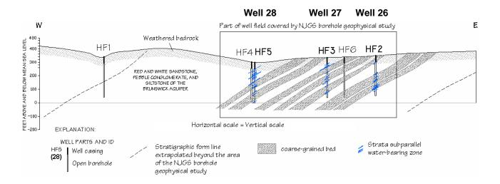
**Figure 2D2.** Hydrogeologic sections (above) based on geophysical logs for wells 26 through 28 showing the vertical distribution of hydraulically-conductive features and water-bearing zones in red and gray sandstone, conglomerate, siltstone and mudstone. Depth values are feet below land surface. The map trace for the hydrogeologic cross section (below) shown on figure 2D1.
